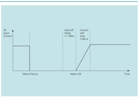
Figure 3. Rectifier soft start
