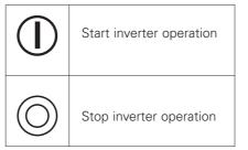
The control shall incorporate a safety feature to prevent inadvertent operation yet still allow for rapid shutdown in the event of an emergency. To stop the inverter the user must press and hold the Stop button for two seconds. An audio alarm shall be activated during this delay time.
