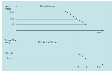
Figure 2. Rectifier behaviour during reduction of the commercial AC source.
