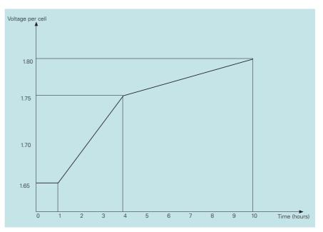
Figure 4. End-of-discharge voltage in relation to discharge time
