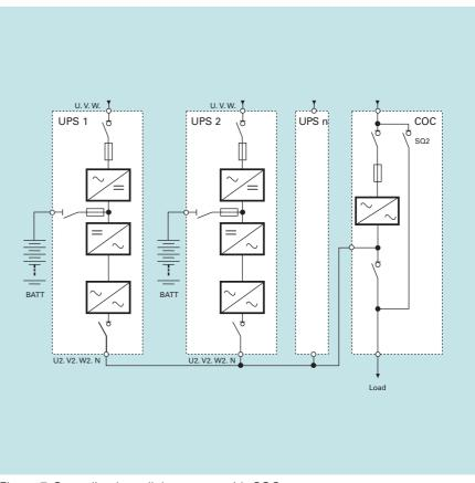
Figure 7. Centralised parallel systems with COC
